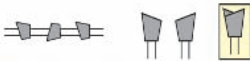
ATAF (Alternate Top Alternate Face) - Extra sharp cutting tips reduce load on saw. - Face beveling diverts cutting load left and right, instead of straight on. - Creates a better shearing action - especially in cross-grain, natural wood.
