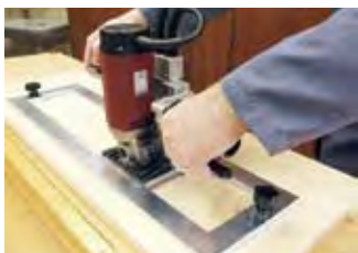
Milling jig for Minispot patching rods
