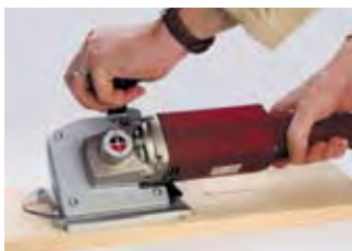
Planing protruding patch
