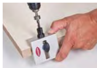
2. Slide the drill jig into the groove and drill the access hole
