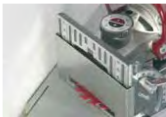
Cutting expansion gaps
