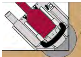
45° cut into the corner
