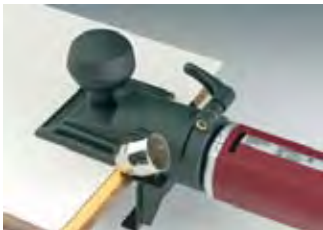
Trimming of surfaces
