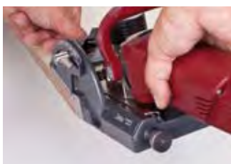
1. Cut the profile groove with the Lamello Zeta
