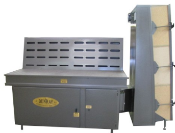
Downdraft table with Backdraft, HEPA Filter bank, and HDPE Plastic top
