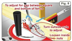
the bracket as shown in **Figure 8**, and then tighten the other outside nut by the same amount in the same direction against the rear leg. Alternate this 1/6 turn procedure between the two nuts until the fence is perfectly square to the table DO NOT TURN THE SET SCREW and DO NOT over tighten the nuts. It usually takes less than 1 full turn of the nuts to square your fence to the table.
