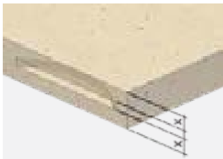
Adjust groove to middle
