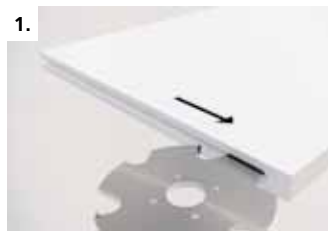
Groove with Zeta P2 / CNC
