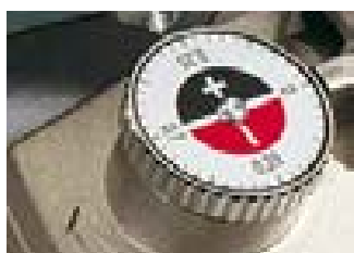
High-precision cutter adjustment
