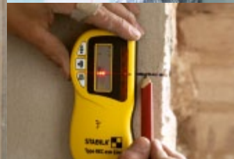
Line receiver REC 210 Line contained in the complete set (17283/1).
