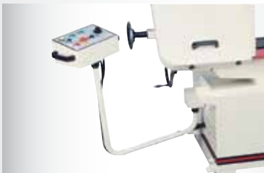
SWING AWAY CONTROL PANEL
