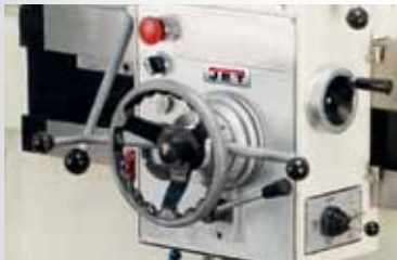
HANDWHEEL FOR HORIZONTAL GEARBOX TRAVEL
