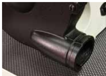
CAST IRON GUARDS AND DUST CHUTES
