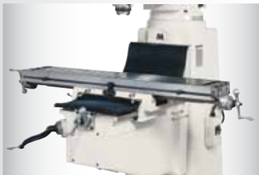
HARDENED & GROUND 10X54" TABLE CERTIFIED TO 52C ROCKWELL HARDNESS
