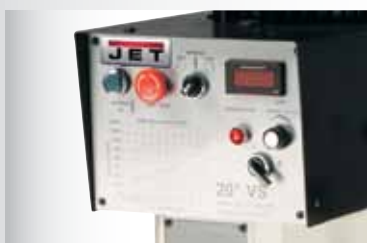
DRILLING CHART ADDED FOR OPERATOR EASE OF USE
