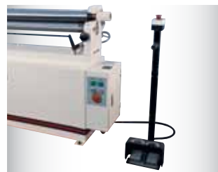
EASY TO USE FORWARD AND REVERSE FOOT PEDAL WITH E-STOP
