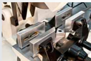
SPLIT SOFT JAWS WILL NOT MARR SOFT CUTTING MATERIALS
