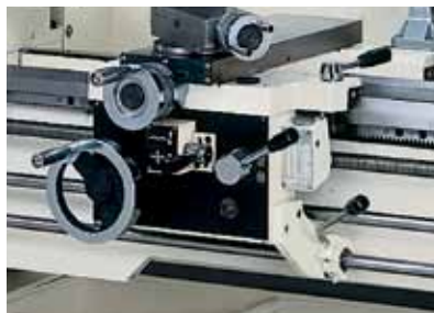
COMPOUND AND CROSS SLIDE HAVE BACKLASH ADJUSTMENT
