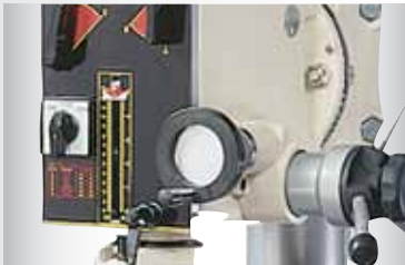
FINE FEED ADJUSTMENT KNOB IN EASY TO REACH LOCATION
