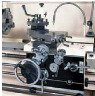
CARRIAGE FEATURES ONE-SHOT LUBRICATION AND TURCITE B ON SLIDING SURFACES
