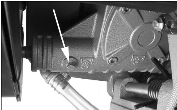
Figure 11-1: gear box drain
