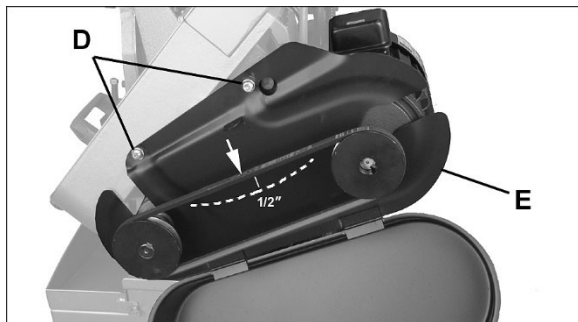
Figure 5-4: installing belt and pulley cover
