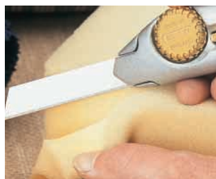
NON-SEGMENTED BLADE — IDEAL FOR CUTTING FOAM.
