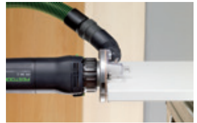
Rounding plastic or solid wood veneer.
