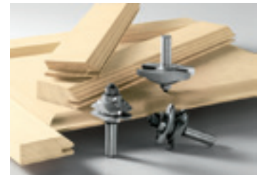
Profile/groove cutter HW with ball bearing guide, shank 8 mm HW s = 8
