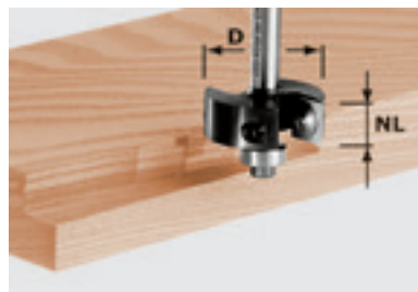
Turning plate rebating cutter with ball bearing guide, shank 8 mm
