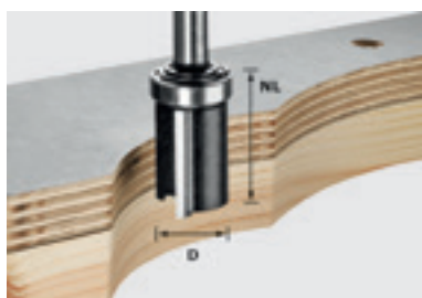
Edge trimming cutter HW with ball bearing guide, shank 8 mm HW s = 8
