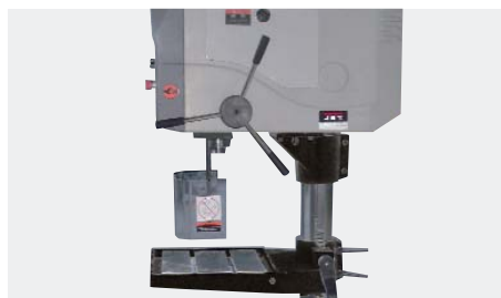
T-slotted table, precision design with rack and pinion table riser
