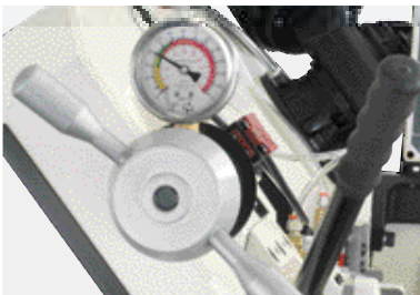
Hydraulic blade tension scale and blade breakage detection
