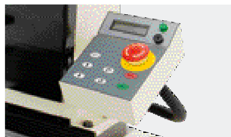
Control panel with digital display for spindle speed
