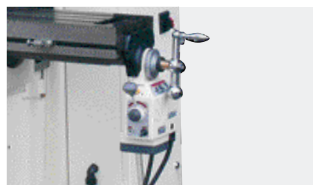
Automatic x-feed 0–900 mm/min, with limit switches and rapid feed button
