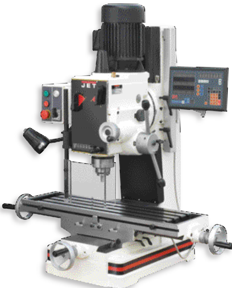
Glass scales for X-, Y- and Z-Axis (JMD-45PFD)
