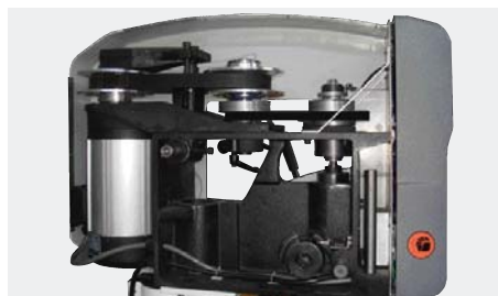
Variomatic, 2/4 pole motor, stepped pulley
