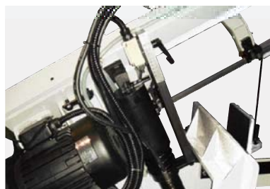
Automatic bow rising after end of cut
