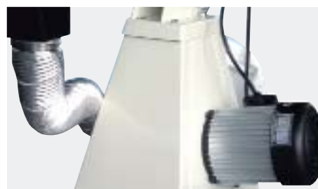
Integrated dust collection system (MBG-75DC)
