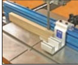
Add a stop to the fence for producing cuts to a repeatable depth, such as cutting tenons.
