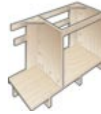
Framed Cabinets (rear view)
