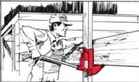
FOR RAISING BEAMS
