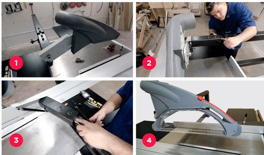
Fig. 1: Attach the saw guard to the frame.
