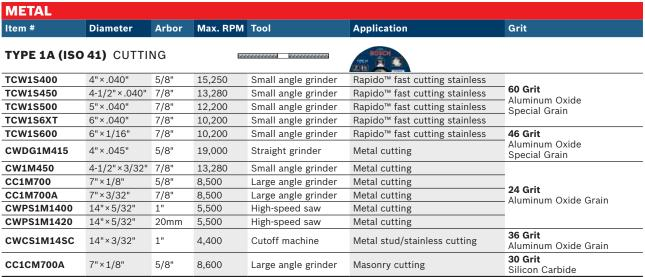
NOTE: All cutting wheels require use of Type 1A (ISO 41) guarding. Abrasive cutoff wheels must be rated at least the speed recommended on the tool label. See page 56 for appropriate metal or masonry cutting guard.
