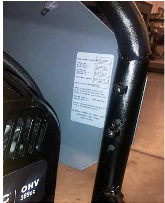
Figure 1: Unit ID Location
