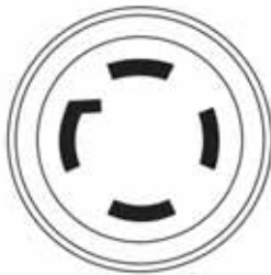
Figure 2-10: 120/240 VAC, 30 Amp Receptacle
