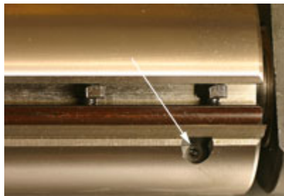
Our controlled chip, three knife cutterhead feature jack screws (arrow, left photo) that make setting precise knife heights very easy. We also include a simple knife-setting jig (right). When the knife is at the correct height, if the first arrow is placed at the end of the outfeed table and the knife rotated under the jig, the jig should move so the second mark is at the edge of the outfeed table.
