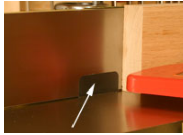
The fence has an insert (left) that prevents scratching the table when it is moved. The operating mechanism (right) allows precise bevel setting and a very stable fence when locked.
