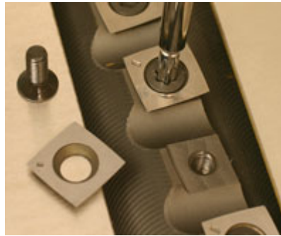
The helical cutterhead (left) uses individual solid carbide cutters, each with four cutting edges that can be "indexed" four times should the first edge become dull. We include five extra carbide cutters, screws and two drivers with the PJ-882HH. One driver is placed in a screw to hold the head steady while the other driver loosens the screw at the cutter to be replaced or indexed.
