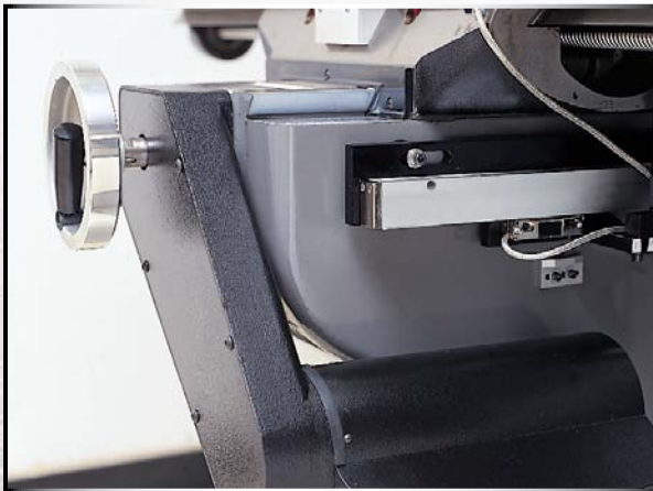
Precision Glass Scales to Provide Better Accuracy, Repeatability, Elimination of Backlash and Much More!
