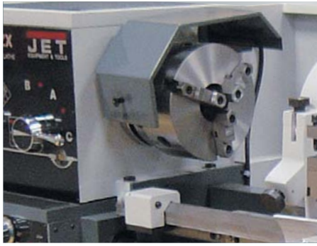
Ø250 mm three-jaw chuck with basic and reversing jaws, chuck guard with limit switch
