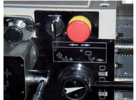
Z-axis rapid feed 5 m/min (GH-2280ZX)
