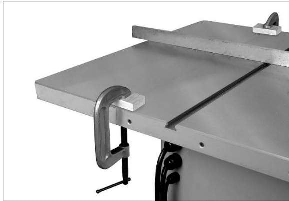
Figure 6-5: leveling extension wings, method 2
