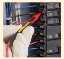
Reduce tip exposure for CAT III testing
